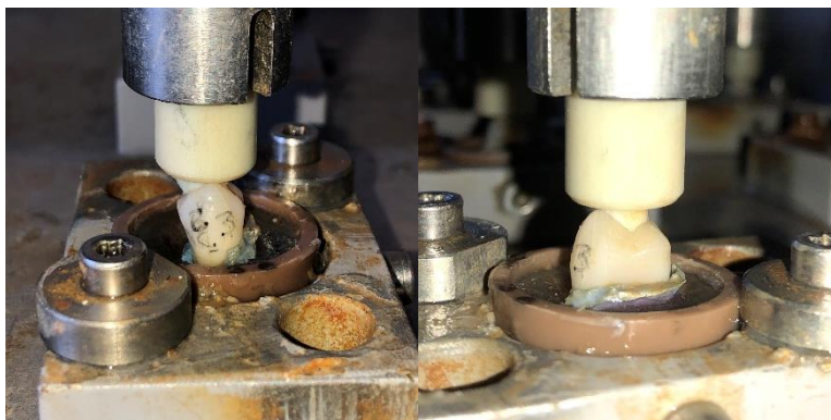
Figure 8 – positioning of the specimens in the pneumatic mechanical cyclus. The antagonist piston of G10 and the tooth touch each other forming a tripodism.
