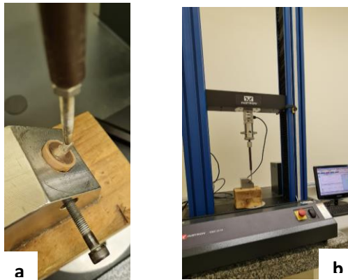
Figure 6. Fracture resistance test on an Instron universal testing machine. a) positioning the sample in the device and
